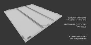
\* Spans and number of stiffeners are calculated based on the cassette size and other factors. Stiffeners are usually fixed with tac welds or structural adhesive (or 3M® Tape).
