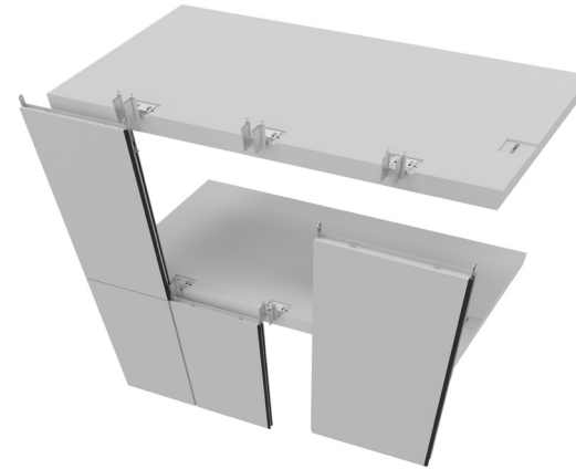
Curtain Wall INSTALLATION - Joint Detail
